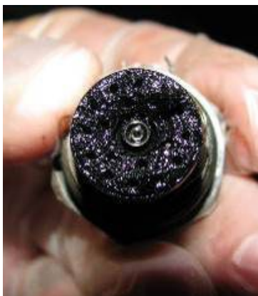
Fuel nozzle (nach Pilot Owner Maintenance)
